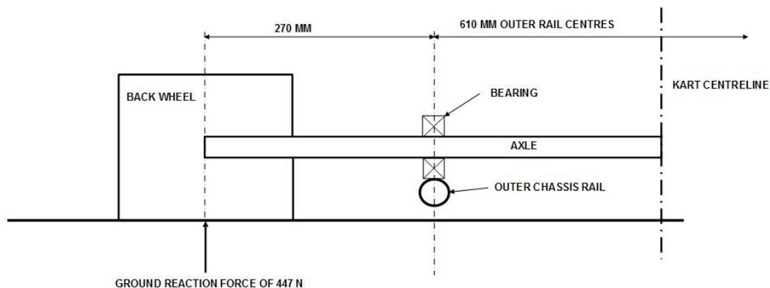
From the above situation, we can compare the stress in the axles and the deflection at the wheel. In doing this, we must acknowledge the following assumptions for simplicity:
