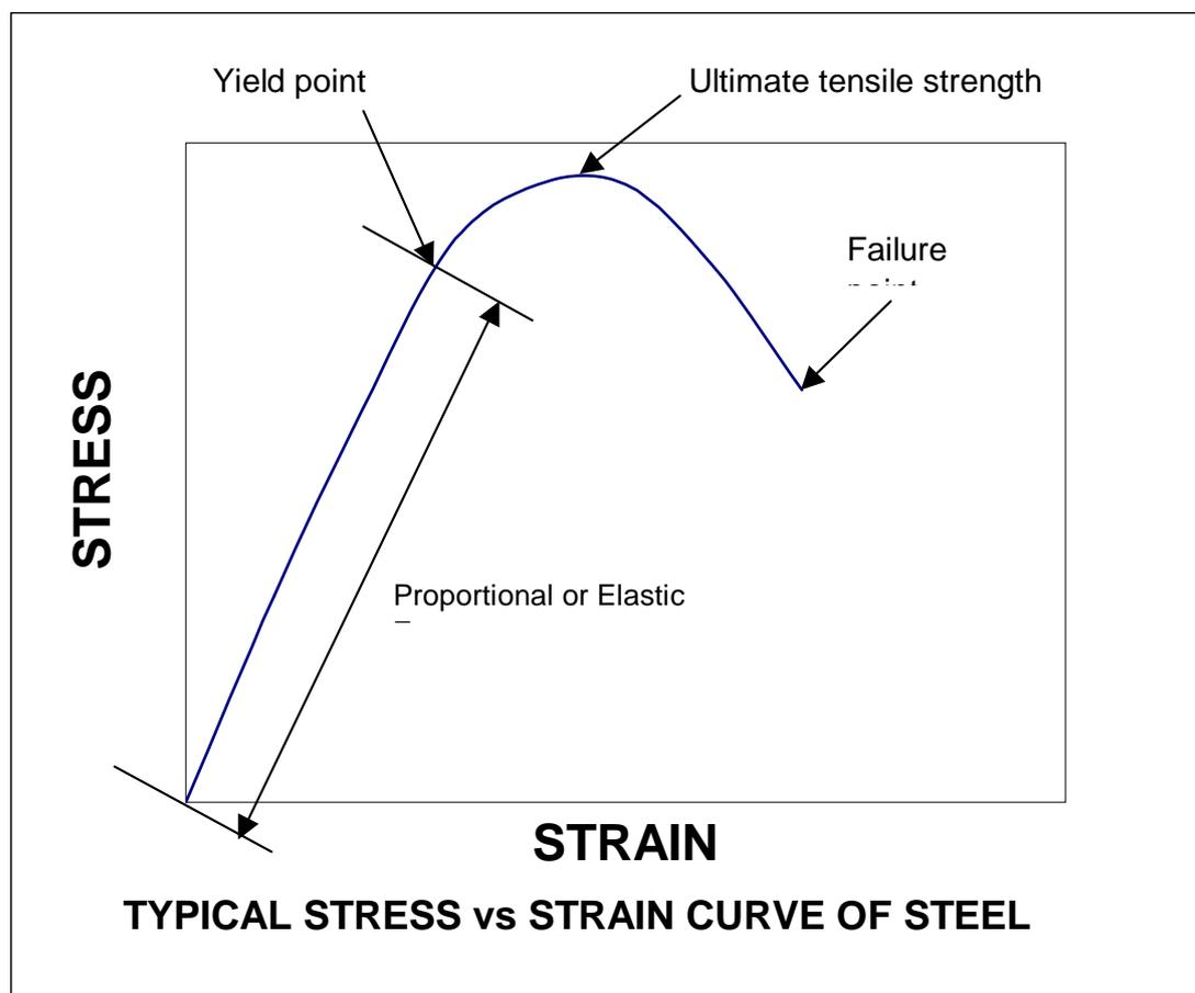
What can be seen from this is that there is a proportional zone of the stress/strain curve where the material acts as a simple elastic spring. It can receive a limited amount of stress (up to the Yield point) and it will deflect and return to its initial shape or length. Beyond the Yield point, the steel will withstand an increasing level of stress until it reaches its Ultimate Tensile Strength. Shortly after this point, the material will fail.
